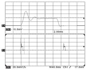
Figure 18: Load current (5A/div) as a function of time when the converter attempts to turn on into a 1 m $\Omega$  short circuit. Top trace (2ms/div) is an expansion of the on-time portion of the bottom trace.
