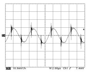
Figure 15: Input reflected ripple current, is, through a 10 µH source inductor at nominal input voltage and rated load current (5 mA/div). See Figure 13.
