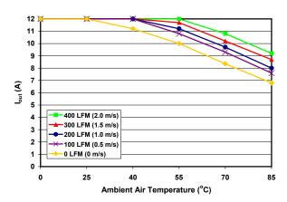
Figure 5: Maximum output power derating curves vs. ambient air temperature for airflow rates of 0 LFM through 400 LFM with air flowing across the converter from input to output (nominal input voltage).
