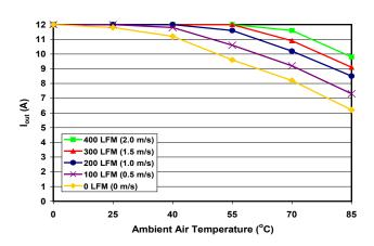
Figure 7: Maximum output power derating curves vs. ambient air temperature for airflow rates of 0 LFM through 400 LFM with air flowing from pin 1 to pin 3 (nominal inout voltage).
