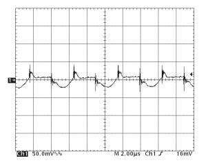
Figure 16: Output voltage ripple at nominal input voltage and rated load current (50 mV/div). Load capacitance:  $1\mu F$  ceramic capacitor and  $10\mu F$  tantalum capacitor. Bandwidth: 500 MHz. See Figure 13.
