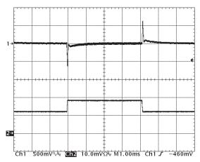
Figure 11: Output voltage response to step-change in load current (50%-75%-50% of Iout(max);  $dI/dt = 0.1A/\mu s$ ). Load cap:  $10\mu F$ ,  $100 \, m\Omega$  ESR tantalum capacitor and  $1\mu F$  ceramic capacitor. Ch 1: Vout (500mV/div), Ch 2: Iout (5A/div)
