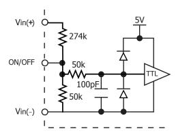
Figure B: Internal ON/OFF pin circuitry
