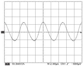
Figure 14: Input Terminal Ripple Current, ic, at full rated output current and nominal input voltage with 10µH source impedance and 47µF electrolytic capacitor (200 mA/div). (See Figure 13)
