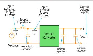
Figure 13: Test set-up diagram showing measurement points for Input Terminal Ripple Current (Figure 14), Input Reflected Ripple Current (Figure 15) and Output Voltage Ripple (Figure 16).
