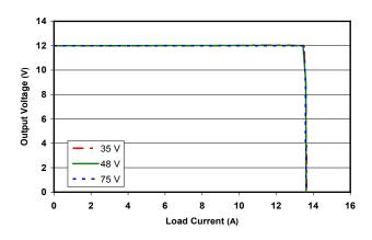
Figure 17: Output voltage vs. load current showing typical current limit curves and converter shutdown pints.
