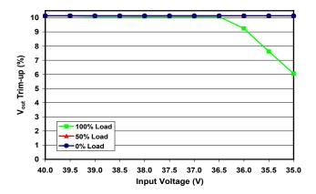
Figure 23: Percentage of output voltage trim-up that can be achieved at various input voltages frm 35V-40V and output loads of 0%, 50% and full load.
