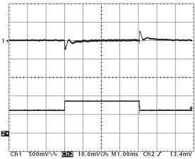
Figure 12: Output voltage response to step-change in load current (50%-75%-50% of lout(max):  $dI/dt = 1A/\mu s$ ). Load cap:  $470\mu F$ ,  $30 \text{ m}\Omega$  ESR tantalum capacitor and  $1\mu F$  ceramic cap. Ch 1: Vout (500V/div), Ch 2: lout (5A/div).
