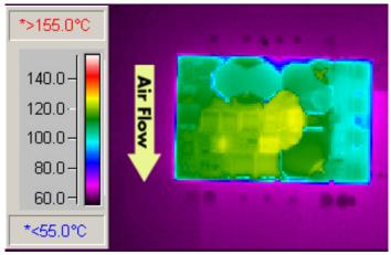
Figure 8: Thermal plot of converter at 11.6 amp load current (139W) with 55°C air flowing at the rate of 200 LFM. Air is flowing from pin 1 to pin 3 (nominal input voltage).
